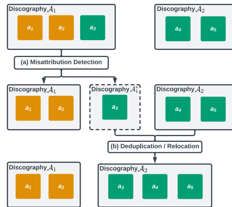
Figure 1: System Overview: (a) Misattribution detection is performed on each discography \mathcal{A} . The misattributed release a_3 is split out from \mathcal{A}_1 into sub-discography \mathcal{A}_1^* . (b) All (sub-)discographies are considered for deduplication; \mathcal{A}_1^* is merged into \mathcal{A}_2 , relocating the misattributed releases into the correct discography.
