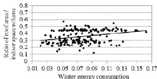
Fig. 2 Winter energy consumption and ratio of roof area to indoor space volume
