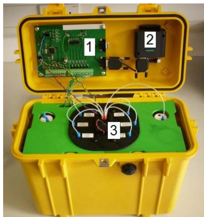
Fig. 2 The prototype phosphate analyser system. (1) Electronics board. (2) GSM modem. (3) Microfluidic chip / detector assembly. The battery, storage bottles, and solenoid pumps are contained within the lower part of the case
