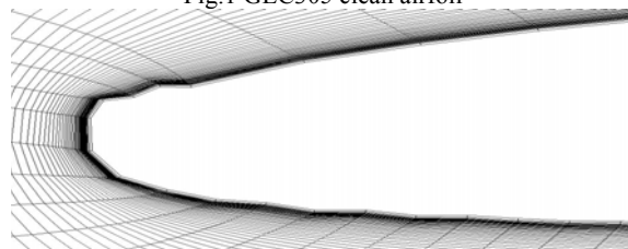
Fig.2 GLC305 airfoil with rime 212 ice shape
