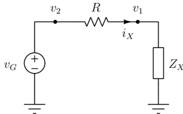
$$i_X = \frac{v_2 - v_1}{R}$$
