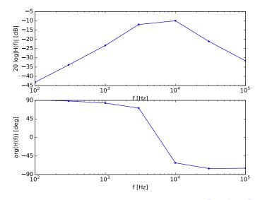
frequency response of the oscilloscope input filter
