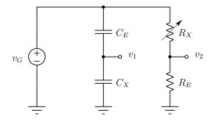
De Sauty bridge with potentiometer, angle versus capacitance, no computing, assemble and measure, protoboard
