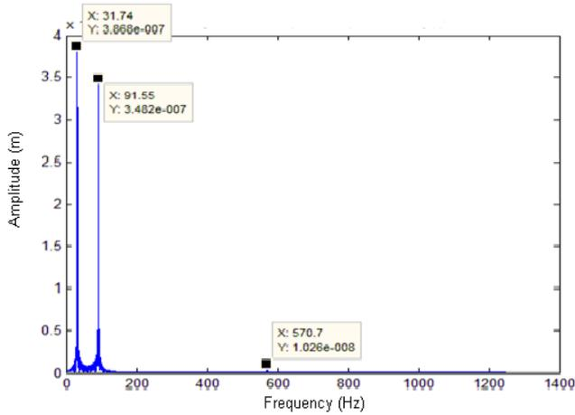
Fig. 6 FFT diagram of the intact beam using ABAQUS modelling exposed to cosine force
