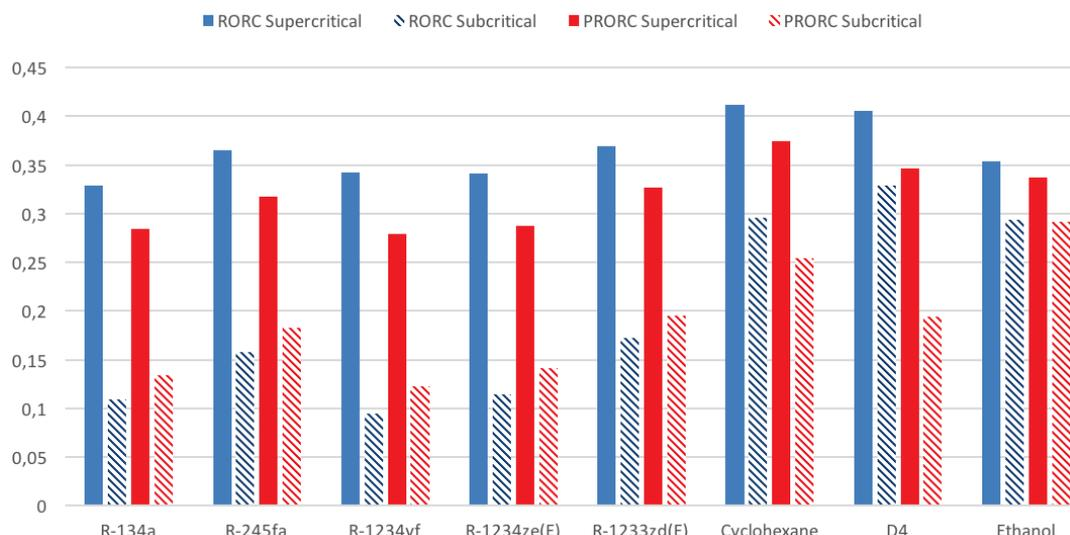
Fig. 3 Thermal efficiency for RORC and PRORC
