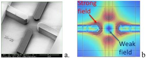
Fig.1. Quadrupole microelectrode sensors implemented in BiCMOS technology (a), electric field gradient on the quadrupole electrode structure (b).
