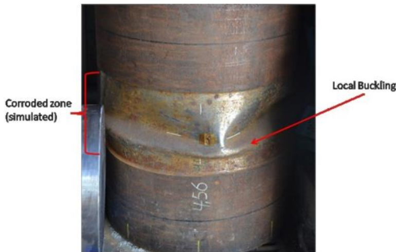
Figure 3-3. Local buckling produced by external corrosion on casing [30]
