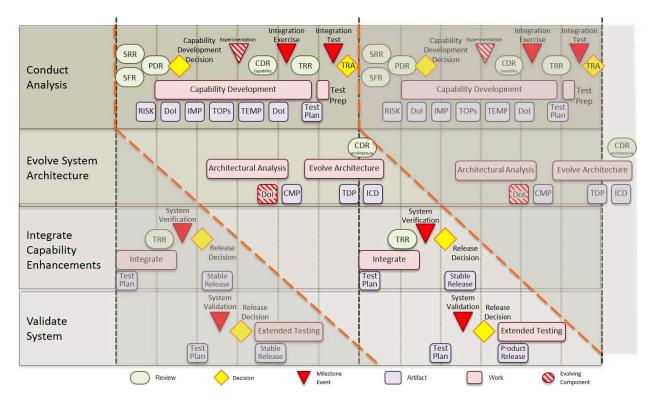
Figure 5. SSC Pacific Evolutionary Systems Engineering Strategy Chart illustrating the major activities and artifacts for the development, assessment, and integration of new and maturing technologies into the baseline autonomous system.
