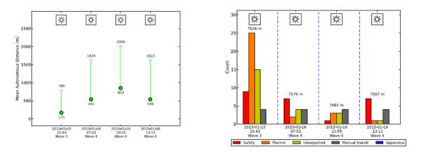
Figure 6. Experimental results over two consecutive waves showing 4x improvement in mean distance traveled and 85% reduction in the number of operator interventions.
