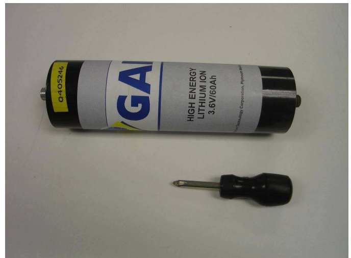
Figure 2. GAIA HE-602050 60AH Lithium Ion Cell
