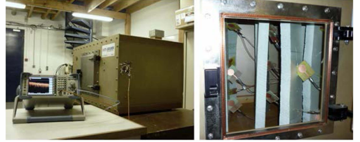
Fig. 3. Picture of the reverberating cell used for this experiment, connected to a vector network analyzer (left). 21 UWB probes are randomly set in the cell to get a 1 \times 20 passive device (right).
