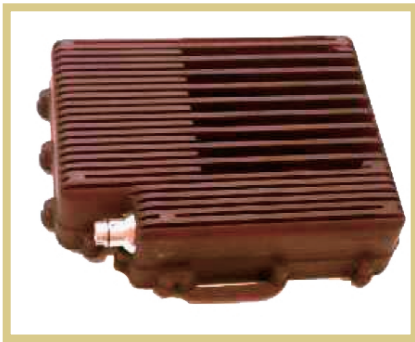
Figure 5. Land Warrior's computer subsystem.
