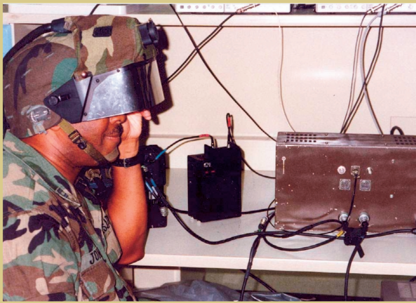
Figure 2. Testing and aligning the SIPE helmet display with the Soldier's Computer in July 1992. The visor reduced ambient light and was a flip-up, flip-down display. It also provided ballistic and laser protection. The right-mounted sensor on the helmet's top was an image intensifier for night vision capabilities. The large brown case is the computer-radio-GPS unit.
