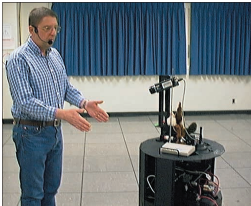
Figure 2. A researcher interacts with Coyote, one of the mobile robots, using natural language and gestures.
