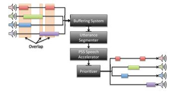
Figure 1. Architecture of NRL's concurrent audio serialization workbench (CASW). Content that overlaps in time on concurrent radio circuits is indicated on the left. Individual circuits are buffered and partitioned into utterance segments. Utterances are then accelerated and presented serially to the listener in a prioritized manner (e.g., first-come-first-serve). AFRL's MMC system (not shown) spatializes the resulting output with a virtual audio engine and provides a speech-to-text display.
