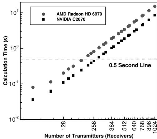
Fig. 1. Plot of total ITM (Longley-Rice) calculation time versus number of transmitters/receivers. The 0.5 second line represents the maximum time allowed for real-time computations.
