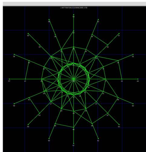
Fig. 4. 16 Outer Nodes Communicate through a Central Node
