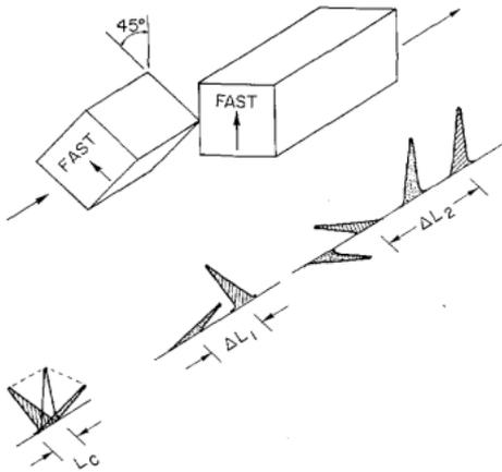
Fig. 3. Model for depolarization in a Lyot depolarizer of broad-band light with coherence length  $L_c$ .  $\Delta L_1$  and  $\Delta L_2$  are the group delay differences experienced in the first and second sections, respectively. For depolarization we require  $L_c \ll \Delta L_1$  and  $\Delta L_2 \sim 2\Delta L_1$ . Depolarization is then independent of input azimuth.
