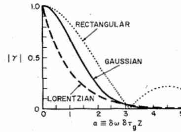
Fig. 2. Magnitude of the degree of coherence for sources with various band shapes.  $\delta\omega$  is the spectral half-width at half-power,  $\delta\tau_g$  the fiber group delay difference, and  $z$  the fiber length.
