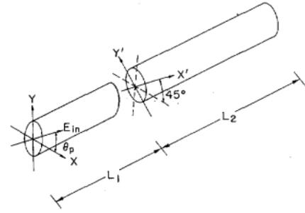
Fig. 1. Model for Lyot depolarizer formed with birefringent fibers.
