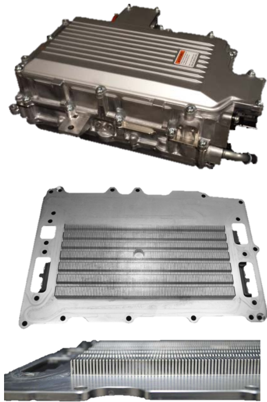
Fig. 3. Pictures of the 2014 Honda Accord power electronics system. The lower images show the cold plate finned structures. Photo Credit: Gilberto Moreno (NREL)
