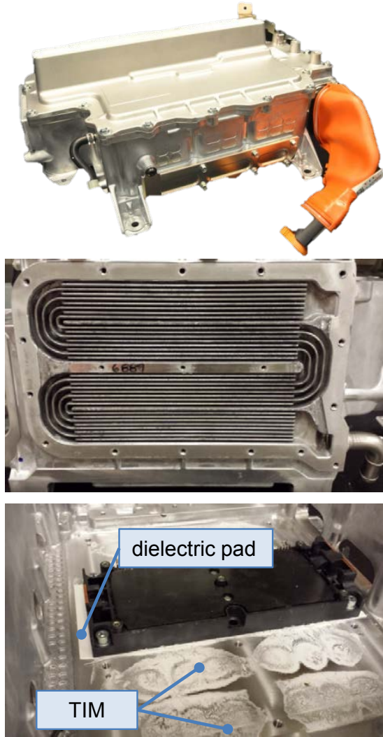
Fig. 1. Pictures of the 2012 Nissan LEAF power electronics system. The middle image shows the cold plate cooling channels. The lower image shows one power module attached to the cold plate. The dielectric pad and TIM layers are shown. Photo Credit: Gilberto Moreno (NREL)
