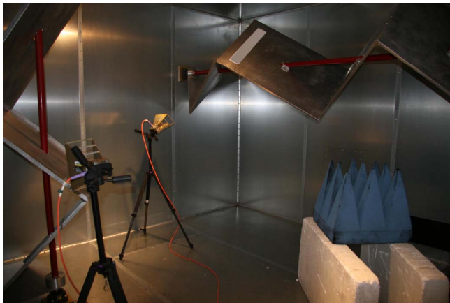
Figure 1. Reverberation chamber used in the measurements with the absorber in position 10.
