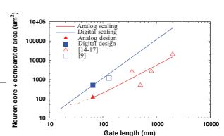
Fig. 7. LIF neuron implementations: analog vs digital neuron evolution according to critical length. A crossover point exists at  $22\ nm$  node
