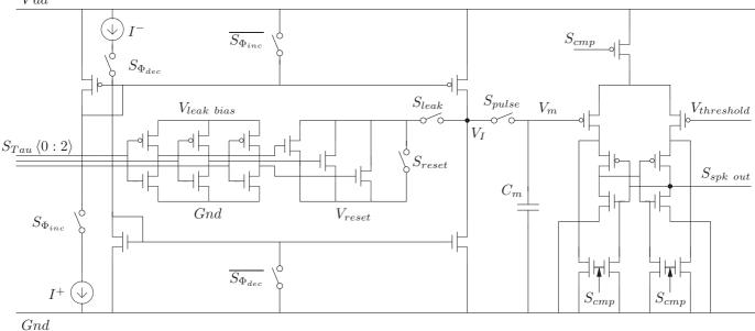
Fig. 2. Analog LIF neuron schematic
