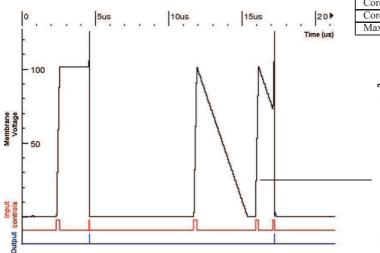
Fig. 6. Simulation of the digital LIF implementation: neuron inputs, output, and membrane potential.
