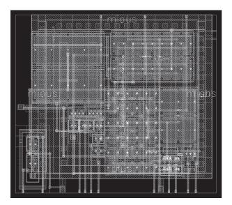
Fig. 4. Analog LIF neuron layout
