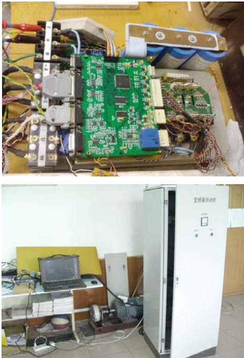
Fig. 2. Physical Self-Made inverter and Test Systems
