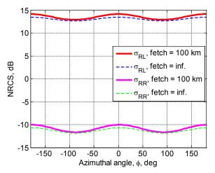
Fig. 6. Comparisons between LHCP ( $\sigma_{RL}$ ) and RHCP ( $\sigma_{RR}$ ) BRCS obtained with the SSA2 for Elfouhaily et al. model and the in-plane geometry for infinite and finite fetch.
