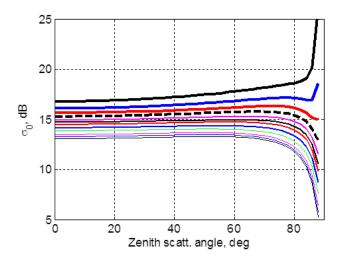
Fig. 1. LHCP BRCS calculated using the KA-GO based on the spectral-derived MSS.
