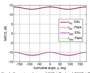
Fig. 4. Comparisons between LHCP ( $\sigma_{RL}$ ) and RHCP ( $\sigma_{RR}$ ) BRCS obtained with the SSA2 for two spectral models and the inplane geometry.
