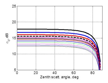
Fig. 2. LHCP BRCS calculated using the KA-GO based on the empirically-derived MSS.
