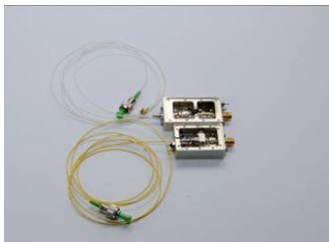
Fig. 3 The optical transmitter (upper) and optical receiver (lower)
