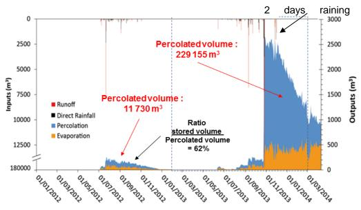
Figure 12. Water budget in the Tummulur tank over period of two years.
