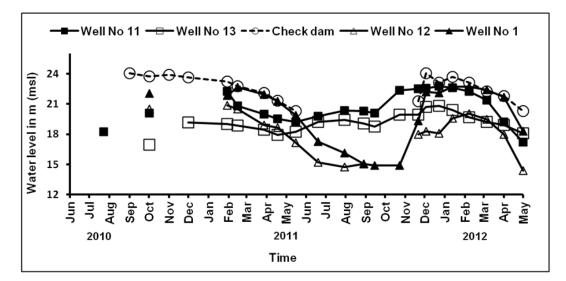
Figure 16. Temporal variation of water level in wells and the Periyapalayam check dam (Parimalarenganayaki and Elango, 2013a)
