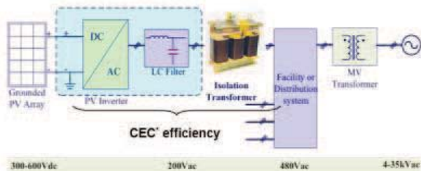
Fig. 1 Typical U.S. commercial scale PV inverter system
