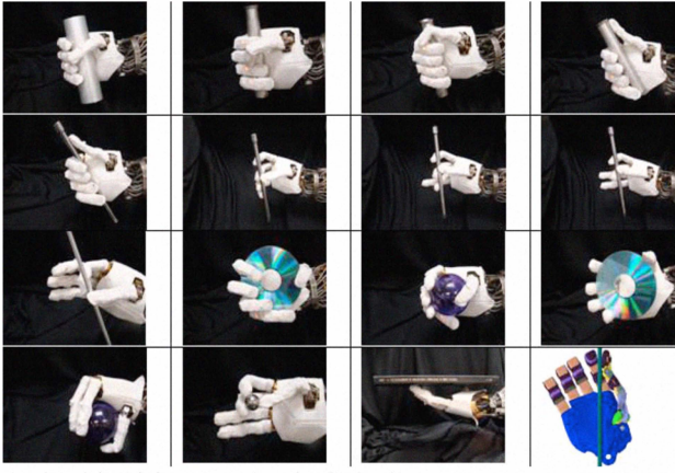
Fig. 2. R2 hand demonstrating the Cutkosky grasp taxonomy
