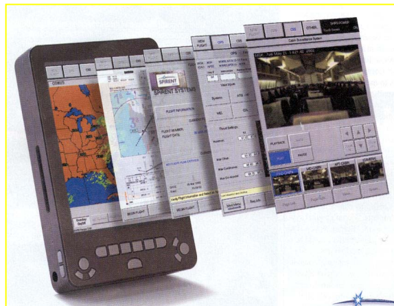
Figure 7. Example of a Portable COTS Multi-Function Display
