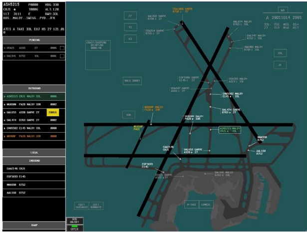
Figure 1. I-TODDS for the ground control position.
