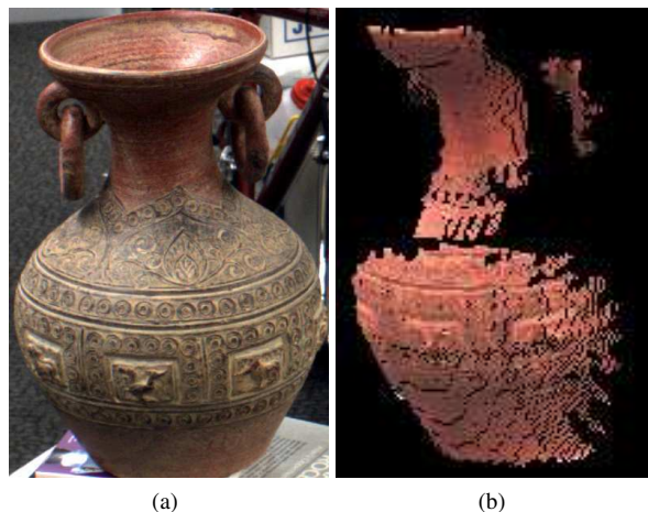
Figure 8: Reconstruction results for a textured object. (a) a pot, (b) the reconstruction after texture mapping.
