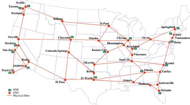
Fig. 2. Physical topology for Sprint network [4]. Each edge in the graph represents optical fibers. The PoP nodes are marked with green box.
