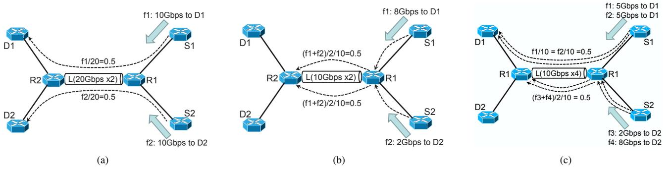
Fig. 4. An illustration of preferred lightpath layout. (a) router capacity is the bottleneck; (b) wavelength capacity is the bottleneck; (c) both router and wavelength capacity are bottlenecks.
