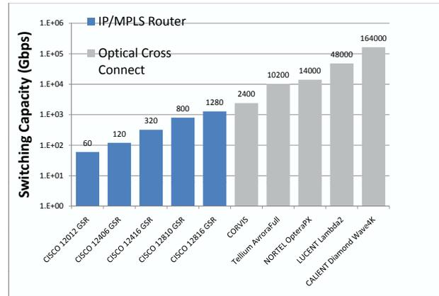
Fig. 3. Comparison of OXCs and routers in term of switching capacity. Information in this figure is collected from [1] and manufacturer web sites based on data from 2006.
