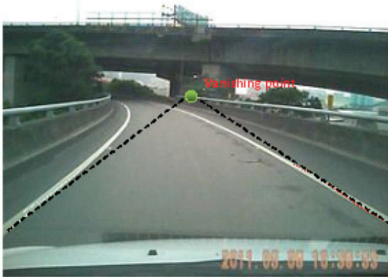
Figure 8. the vanishing point does not match the road trend
