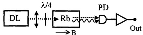
Figure 2: Basic Raman scheme. DL: diode laser, PD: photodiode.
