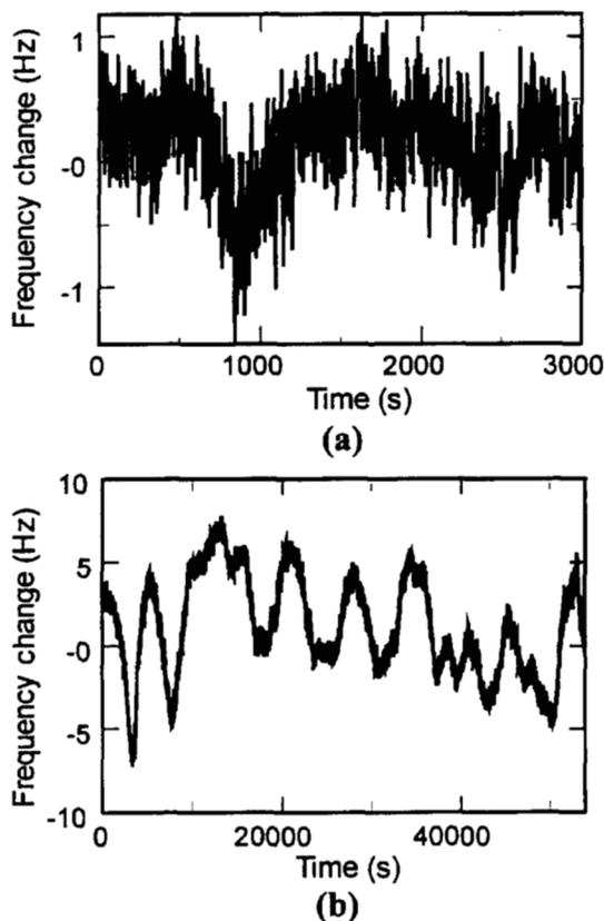
Figure 6: Oscillator frequency change as a function of time. (a) short-time data, (b) long-time data showing thermally-driven fluctuations.
