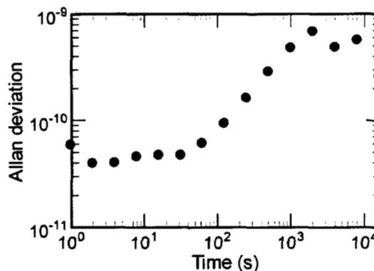
Figure 7: Allan deviation of external oscillator configuration.
