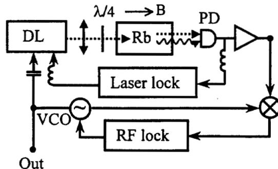
*Figure 5: External oscillator configuration. VCO: voltage controlled oscillator*
