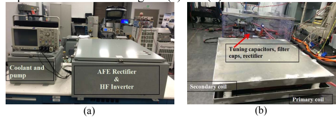
Fig. 16. Grid side unit enclosed in a box with the cooler (a) and primary and secondary coils, tuning capacitors, and vehicle side rectifier and filter.
