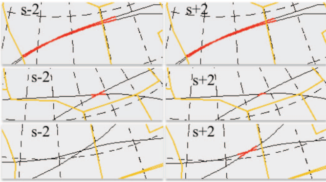
Fig. 13. Examples of conflicts recorded for different forecast wind scenarios, “s-2” (left column) and “s+2” (right column). Trajectory pairs: from EBBR to KEWR and from EDDF to KCLT (top); from EHAM to KMSP and from ESSA to KEWR (middle); and from KEWR to ENGM and from KORD to LIRF (bottom)
