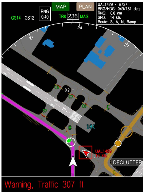
Figure 3. AMM Showing Warning Alert
