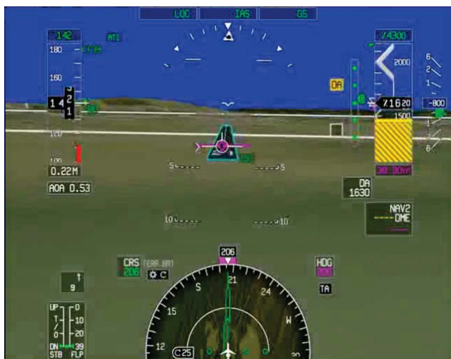
Figure 3. PFD with SVS Image Showing Terrain and Depicting a Runway at 150 ft DA
