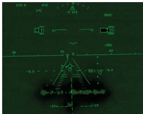
Figure 7. Combined HUD/EVS Image Recording
