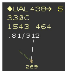
Figure 4. Prototype DSR Data Tag with Trial Planning Portal (Arrow), Speed Advisory, and Predicted Conflict in 5 Minutes
