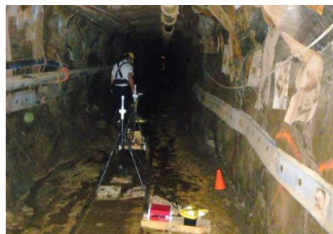
Fig. 1. Radio propagation measurements in an underground silver mine
