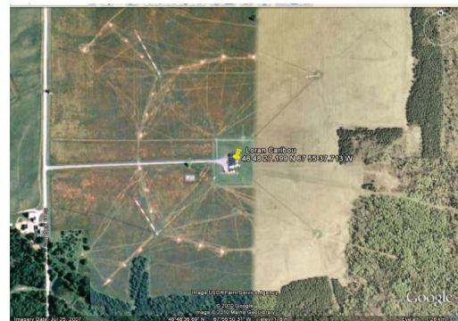
Figure 2. Plan view of Caribou SLT antenna.
