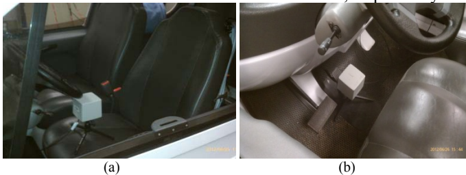
Fig. 15. Magnetic field measurement device locations: driver seat (a) and floor board (b).
