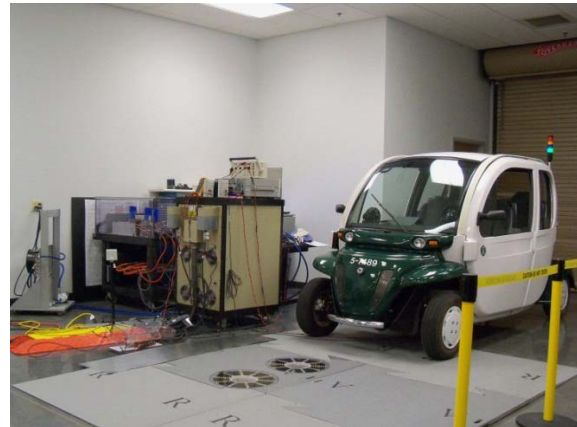
Fig. 7. In-motion wireless vehicle charging system setup.
