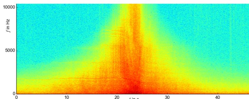
Figure 2: Spectrogram showing the sound pressure level as function of time and frequency.
