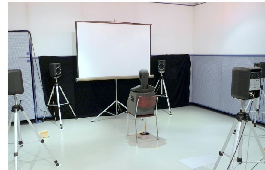
Figure 5: Sound reproduction setup of a previous experiment at Empa. The setup was used in an experiment to determine what Ambisonics decoding strategy to use considering how the head of the listener perturbs the sound field.
