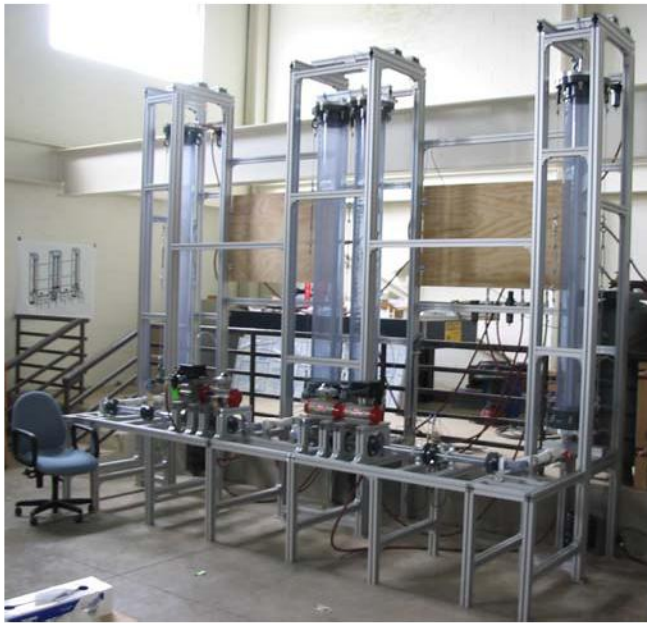
Figure 10 – Photograph of simulated propellant feed system.
