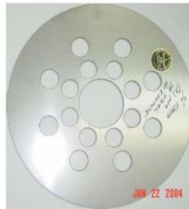
Figure 9 – Balanced Flow Meter (BFM) enables precision propellant flow measurement
