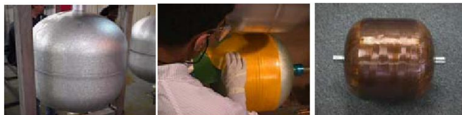
Figure 7 – An example of metallic lined propellant tank overwrapped with composite fibers
