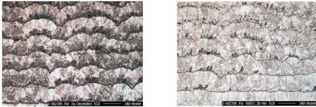
Figure 6 – Micrographs of Engineered EL-Form Re in as-deposited (left) and annealed conditions
