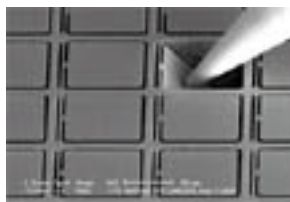
Figure 10 – Close-up of a prototype JWST micro-shutter array. Light shields that mask gaps around the periphery of each shutter are removed for clarity.
