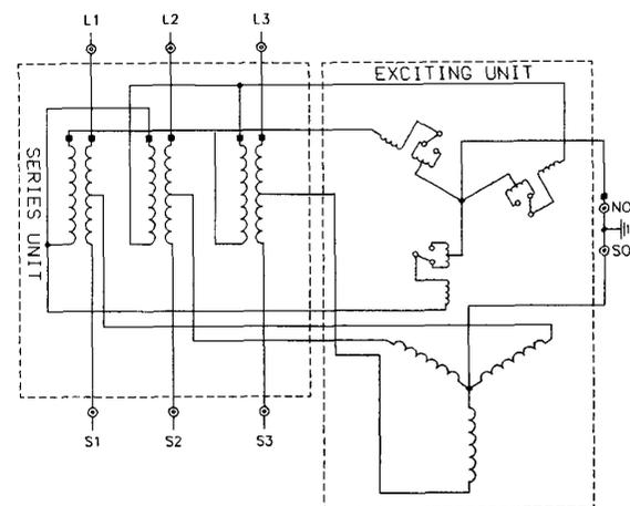
FIGURE 1. PHASE-SHIFTING TRANSFORMER WITH LOAD-TAP CHANGER
