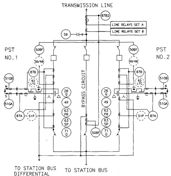
FIGURE 3. PARALLEL PST SWITCHING AND PROTECTION.
