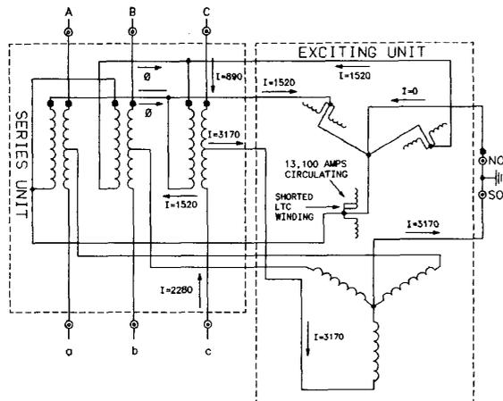
FIGURE 4. FAULT CURRENTS IN THE PHASE-SHIFTING TRANSFORMER
