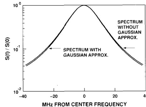
Fig. 2. Field spectrum for a laser with a 7-MHz natural linewidth and  $k = 2 \times 10^{12} \text{ Hz}^2$ . The lower curve is the result obtained using a Gaussian approximation for the field spectrum due to  $1/f$  frequency noise.
