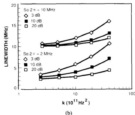
Fig. 11. Linewidth versus  $k$  determined from 3, 10, 20 dB widths of the self-heterodyne lineshape for 2- and 10-MHz Lorentzian linewidths, (a) delay =  $0.5 \mu\text{s}$ , (b) delay =  $50 \mu\text{s}$ .
