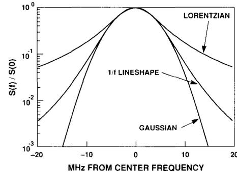
Fig. 7. Normalized self-heterodyne lineshape due to  $1/f$  alone compared to Lorentzian and Gaussian curves with the same 3 dB width (shown for comparison) ( $k = 2 \cdot 10^{12} \text{ Hz}^2$ , delay = 1  $\mu\text{s}$ ).
