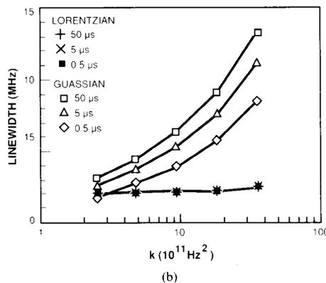
Fig. 12. Lorentzian and Gaussian components estimated from Voigt fitting of self-heterodyne lineshape for delays of 0.5, 5, and 50  $\mu\text{s}$ . (a)  $S_n/2\pi = 10$  MHz. (b)  $S_n/2\pi = 2$  MHz.
