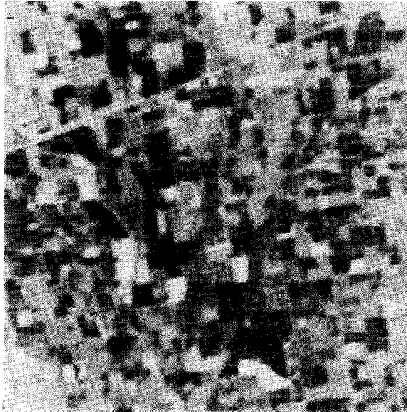
Fig. 2. Temperature values corresponding to Fig. 1. The picture is less sharp due to the 120-m resolution of the thematic mapper thermal IR channel. In this paper high radiances (high temperature) are brighter, while darker areas are cooler. These darker areas correspond to vegetation (compare with Fig. 1).
