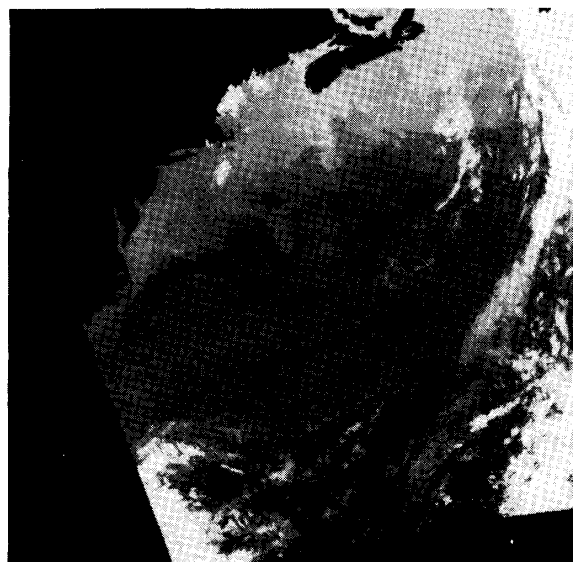
Fig. 1. NOAA-7 AVHRR image showing sea surface temperatures in the Gulf Stream region for April 28, 1983. The image is AVHRR channel four with a spectral bandpass of 10.5 to 11.5 \mu\text{m} . The image is subsampled to a Mercator projection at 4 km/pixel resolution.
