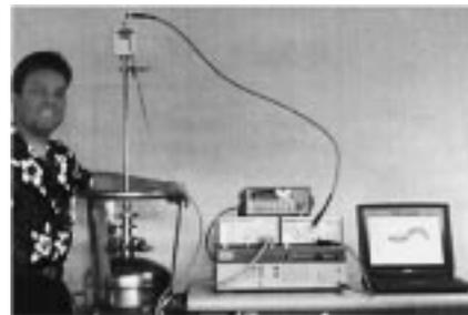
Fig. 5. Programmable voltage standard system. The low-thermal probe is in the Dewar at left. The electronics in the middle (from top to bottom) include a digital voltmeter, dc bias electronics, computer, and microwave source. The system is fully automated.
