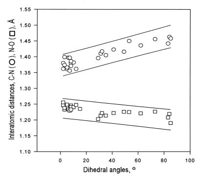
Fig. 3. Distribution of bond lengths (C–N, open circles; and N–O, open squares) versus dihedral angles of individual nitro groups in various salts of trinitromethane (literature data).
